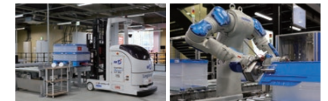
Unmanned forklift system
