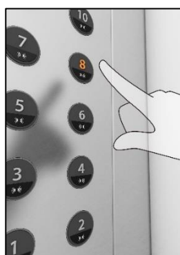
Contactless buttons (infrared beam)
