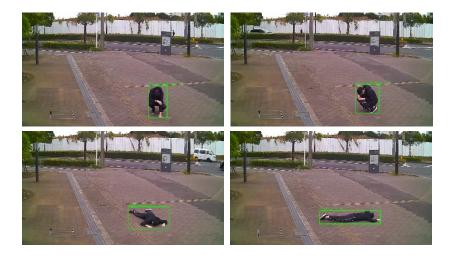
Examples: Detection of a person collapsing or crouching in an image (Images provided by Neural Pocket) Note: There is no guarantee that the incident detection functions of the AI built into the camera will detect the target incident 100% of the time.
