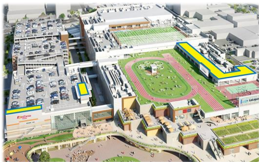
Yellow highlights indicate where solar panels will be installed
