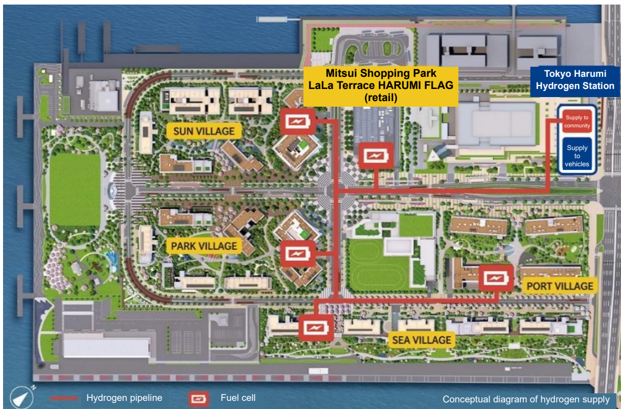
Conceptual diagram of hydrogen supply
